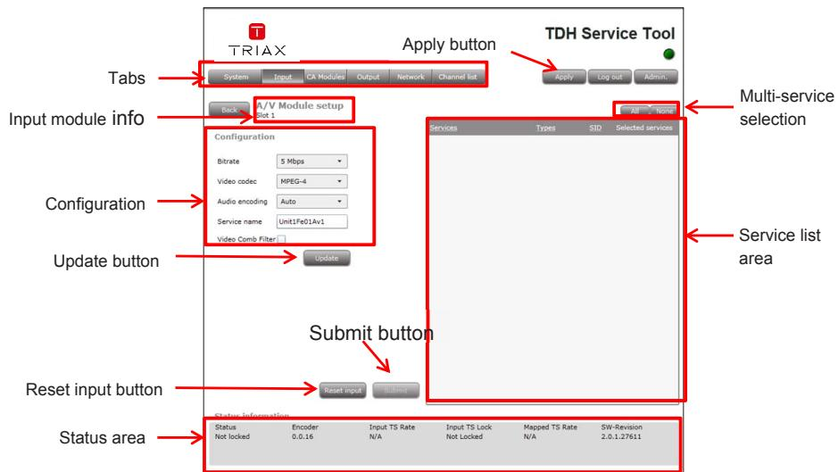
Default values are displayed when the configuration tab is opened for the first time.
