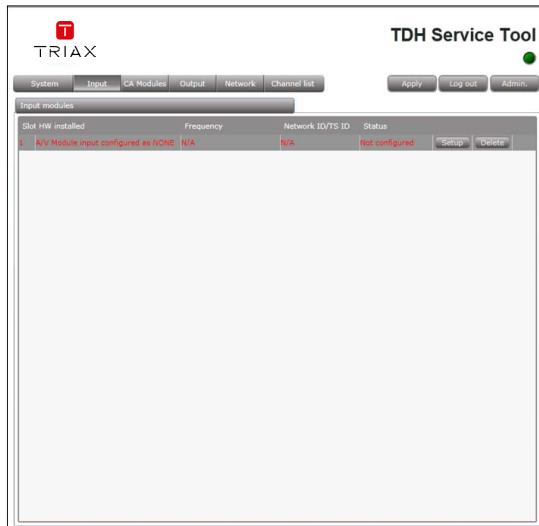
2. Press the **Setup** button of the input module to be configured.
