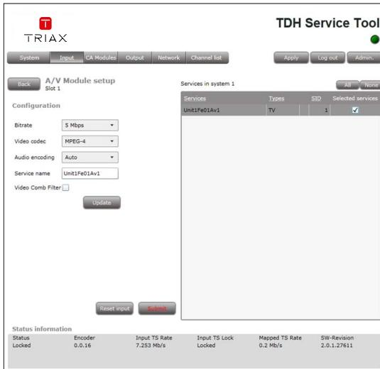
1. Wait for the services list area to be populated with the service(s) that can be delivered from the input module. This can take up to two minutes.
