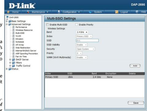
**Encryption:** When you select Open System, toggle between Enable and Disable. If Enable is selected, the Key Type, Key Size, Key Index
