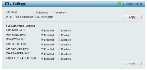
Figure 4.85 – Security > SSL Settings - Enable
