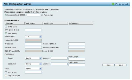
Figure 4.107 - Add Access Rule - IPv6 TCP
