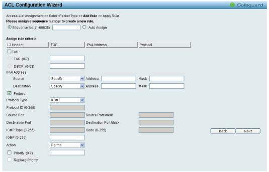
Figure 4.103 - Add Access Rule - IPv4 IGMP
