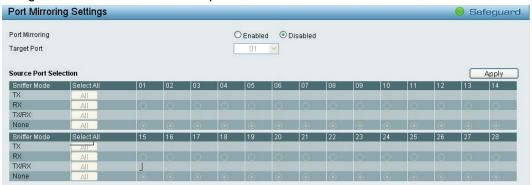
Figure 4.44 – L2 Functions > Port Mirroring
