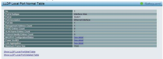
Figure 4.69 – L2 Functions > LLDP > LLDP Local Port Normal Table
