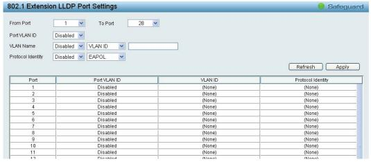
Figure 4.64 – L2 Functions > LLDP > 802.1 Extension TLV Port Settings
