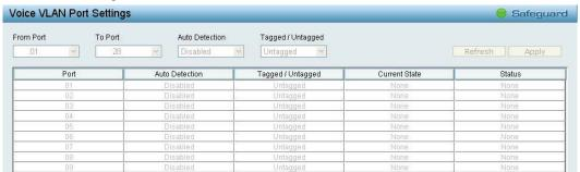
Figure 4.40 – VLAN > Voice VLAN > Voice VLAN Port Settings
