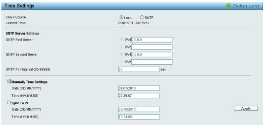
Figure 4.59 – L2 Functions > SNTP > Time Settings
