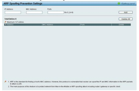
Figure 4.82 – Security > ARP Spoofing Prevention
