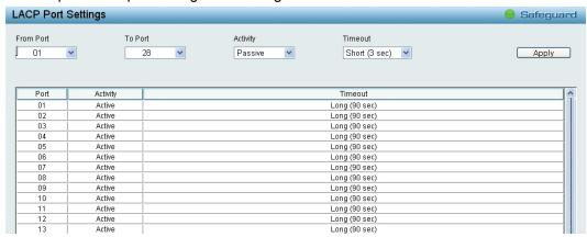
Figure 4.51 - L2 Functions > Link Aggregation > LACP Port Settings
