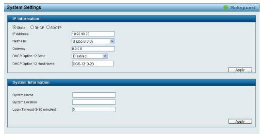
Figure 4.18 – System > System Settings
