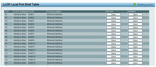
Figure 4.68 – L2 Functions > LLDP > LLDP Local Port Table
