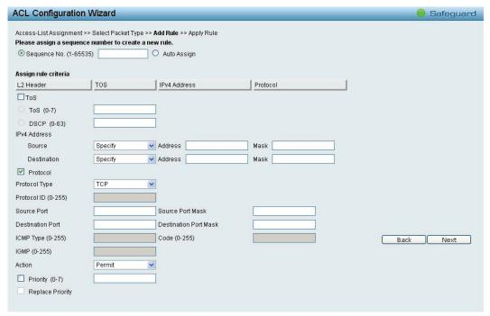
Figure 4.104 - Add Access Rule - IPv4 TCP
