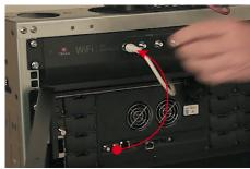
Disconnect the output cable from the TV signal device (shown here with TV out from a headend)
