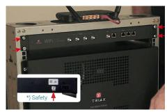
Mount the Controller in 19" rack or on the wall with the brackets
