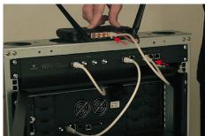
Connect your router or internet modem to the EoC controller with an ethernet patch cable.
