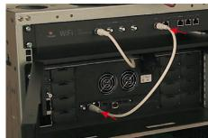
Mount a connection cable to connect your TV signal to the TV in port on the controller.
