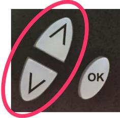
2. Release the UP and DOWN buttons when the LCD shows Reset to Default.
