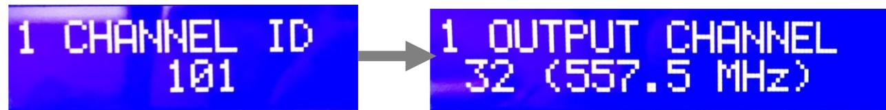
After OUTPUT CHANNEL setting finished, press OK button the screen will show Settings Changed, then go back to the MAIN MENU. (Note: In 60 seconds, the screen will go back to the Channel information)
