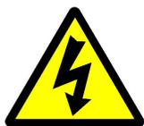
*The presence of this symbol is to alert the installer and user to the presence of uninsulated dangerous voltages within the product's enclosure that may be of sufficient magnitude to produce a risk of electric shock.*
