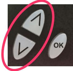
2. Release the UP and DOWN buttons when the LCD shows Reset to Default.
