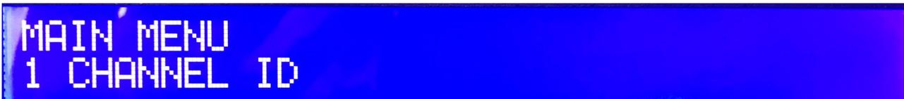
Press OK button to set the desired CHANNEL ID (see Foxtel Channel ID listing at the end of this manual), then press OK to set the desired OUTPUT CHANNEL.
