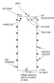
The Kingray Active Taps are specially designed for the distribution of terrerstrial & satellite (Foxtel) services in a multiple dwelling application. They feature high output with adjustable gain and equalisation control.
